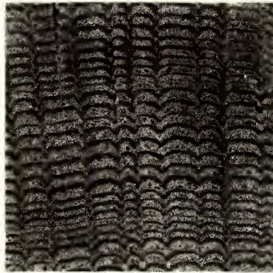
FIGURE 2-74.—Indented rings as seen on a cross section of Sitka spruce. Natural size.
